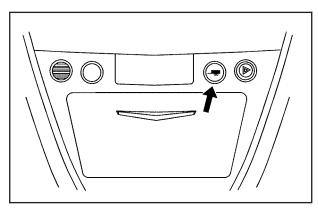
Your vehicle may be equipped with a Tow/Haul mode. The button is located on instrument panel under the climate controls. You should use this feature to assist when towing or hauling a heavy load.
